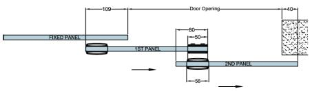
Standard Glass to Glass Overlap is 80mm Glass Protrude by 20mm
